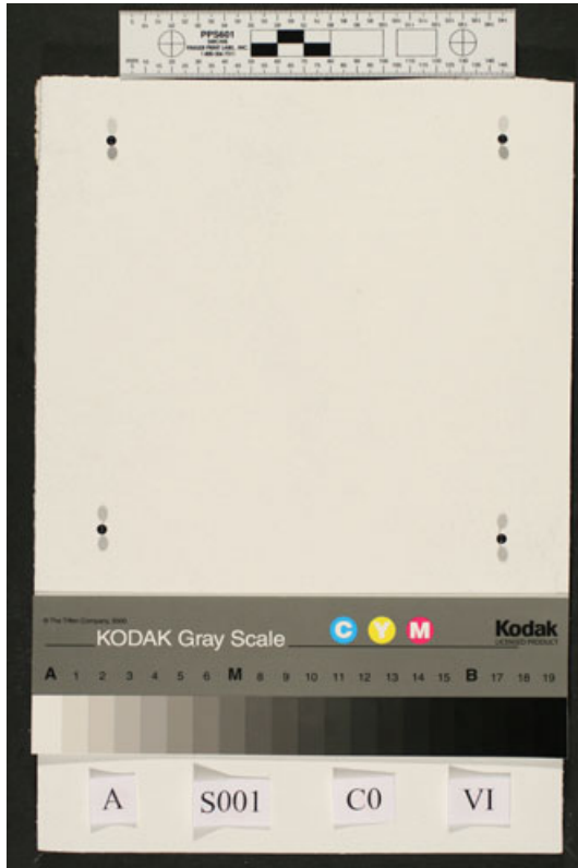
FIG. 2—Layout of samples photographs; (from top to bottom) a linear scale, the plasterboard sample with four black map pins in place, the Q13 test target and the sample number.
